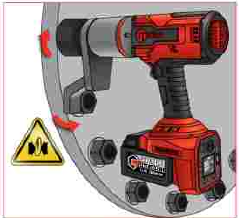
At the above example, 2,000 Nm torque output will result in a reactive force of 2,000 N at a point of 1m from the bolt head reaction of 2,000 N at 0.5 m.
